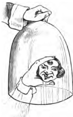
Fig. 114. The squeaking toy, used in a jar of hydrogen.
